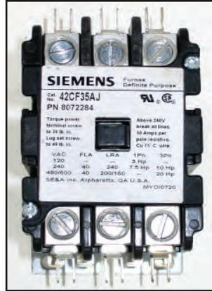
14-17kW Mechanical 50 amp heating contactor. (5-10 ohms coil). Used on domestic units after April 08 until June 2017.
