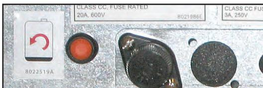
The orange JIB reset button is pressed to reset the system and pressed and held to refill the JIB from the bulk oil system.
