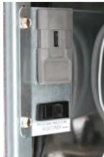
In most instances, the USB port for software updates and the rocker switch for platform resets are in the left column of the left door.
