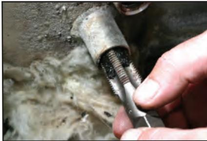
Cleaning the port and clearing the threads with a tap (1/2-14 NPT PN 810-3146) (above) ensures a good seal for the new component.
