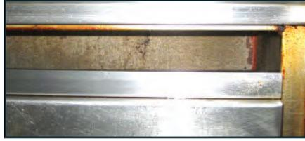
The gap left when a non-Cap-N-Splash fryer is installed in a Cap-N-Splash hood is shown (above).
