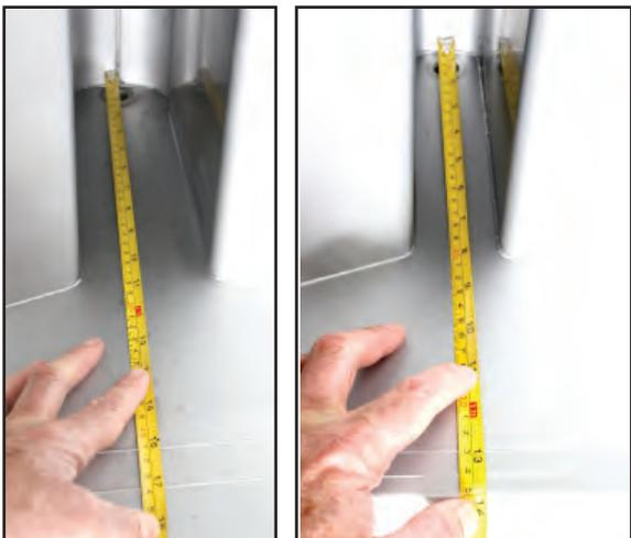
The volume difference is largely in the cold zone of the smaller frypot (right) which is shallower and narrower.
