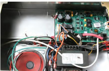
The Smart Interface Board (SIB) is located behind the touchscreen controller.
