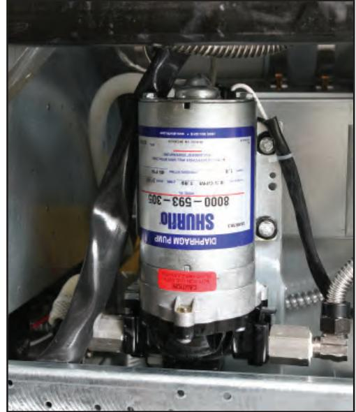
A 24-volt pump moves the oil from the JIB to the frypots. The pump is accessible from the rear of the fryer. It is mounted vertically or horizontally, depending on the space available in the fryer cabinet. If the hose is clogged and pressure builds in the system, a 45PSI pressure switch trips and prevents the pump from running. The system can be checked by removing the hose from the pump to see if the pump resumes running.
