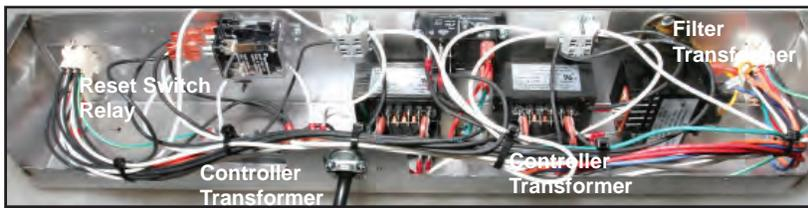
FilterQuick transformer box.
