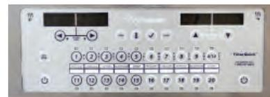
With either controller, verify the presence of system boards with this test, which should be the first step in diagnosing system related failures: failure to filter, failure to top off, etc.
