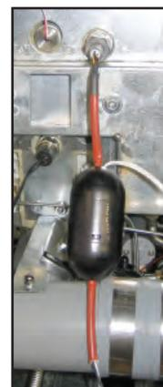
The oil return sensor is controlled by a small board and the electronics inside the egg-shaped device shown above. The board is in the control box; the "egg" is near the probe. The basket lift relay is used to close the coil on the OIB board in the McDonald's unit above. A relay in the box (arrow below) controls the coil on the board in a FilterQuick gas fryer.
