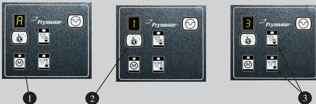
1. Press the M button, which switches the board to manual. The display becomes the number of the vat to be controlled manually.
