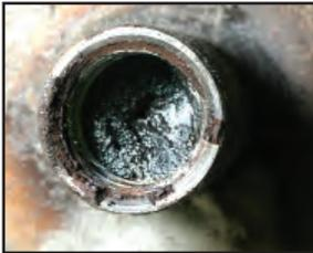
A port is shown clogged with oil (above). Residue left from inadequate cleaning will cause a poor seal on a new component.
