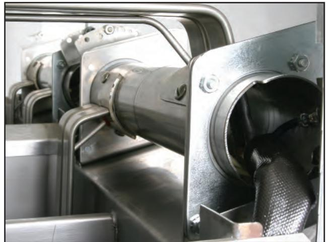
The three-phase wiring, enclosed in a conduit and sheath to meet new UL requirements, enters the rotating tube through an open end. The probe is shielded to reduce RF interference. The temp probe wiring on a replacement element or probe may be wire tied to the outside of the conduit.
