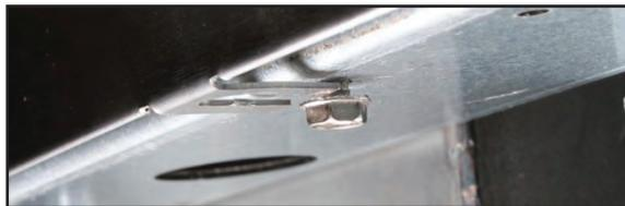
The sides of the fryer are removable. Screws fit into slots on the side panels and bottom (left and above). Loosening them allows the side to be removed to access the gas valve, top off pump.
