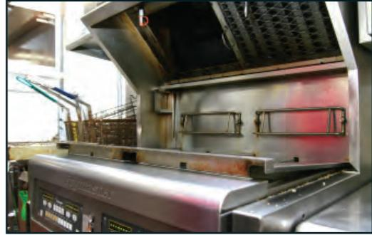
The rim encircling the frypots and attaching to the backsplash is shown raised (above).
