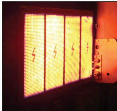
The burner must have an airtight fit to heat efficiently. Insulation strips are wrapped around the burner rails (above) to ensure a good seal. The radiants of a burner glow blue at startup. After approximately 1 minute, a bright orange glow (right above) should appear. If the burner remains blue, there's an improper gas/air mixture.
