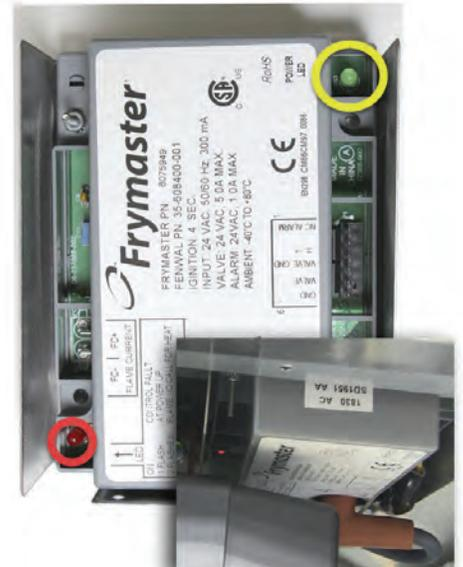
Right module with view of dimmer flashing LED in inset.
