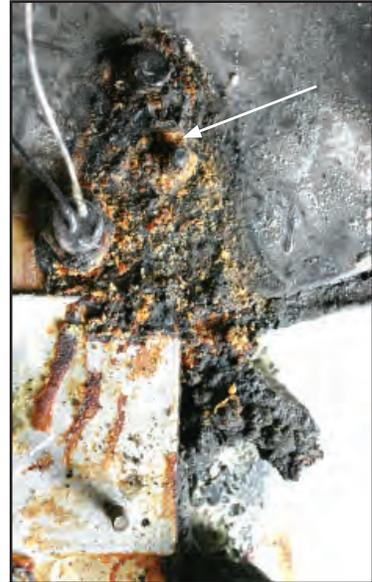
A trail of caramelized oil is visible here, leaking from a service pot plug.
