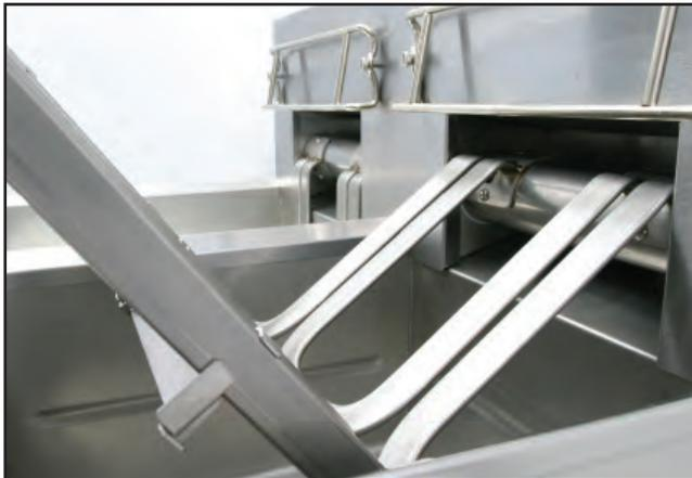
The elements are attached to a horizontal tube, which rotates on bushings.
