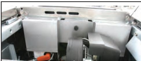
Spark modules on gas units are suspended under the control box. Two screws hold the cover. Two bolts attach the module's box to the bezel above.
