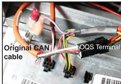
The sensor is wired in series with the CAN bus. The existing CAN cable is disconnected from the second controller from the left and the sensor plugged in. The OQS sensor cable is shown on the right: black terminal to existing CAN; gray to controller and ground.
