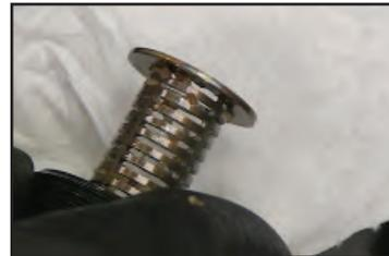
The in-line filter, a line of defence for the sensor and the filter pump, (left) must be cleaned regularly. A month's worth of debris is shown in a clogged filter (center, above). A clean filter is shown right. Slow return of oil to the fry pot can often be traced to a clogged in-line filter.
