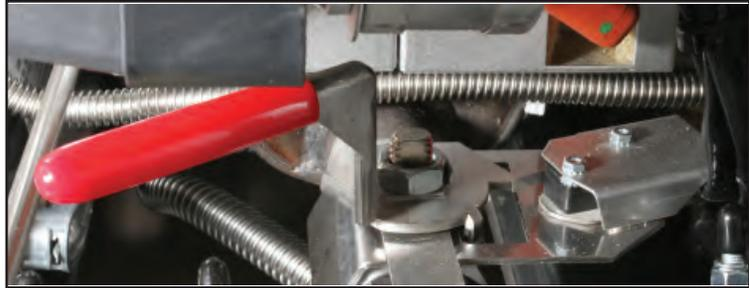
Safety drain switch on H55 drain valve.
