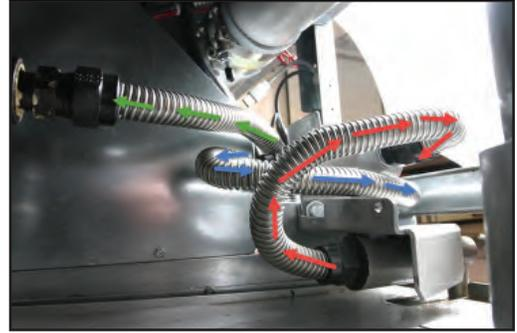
Oil flows from the filter pan (red arrows) to the in-line or pre-filter.
