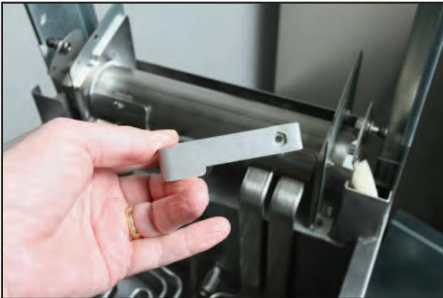
A special wrench (230-4028) is available to capture the element-securing nut inside the tube.
