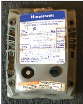
Lack of adequate cooling air can damage spark modules.
