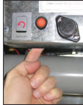
Resetting the power on an electric LOV.
