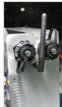
An antenna on the exterior of the FIB is the connection to the store's wireless. Caps on either side of the antenna provide access to LAN and USB ports.
