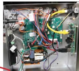
The Filter Interface Board (FIB) is in a box with other components behind the JIB. The box also contains the SUI communication board and power supplies for the top off pump and the communication components.
