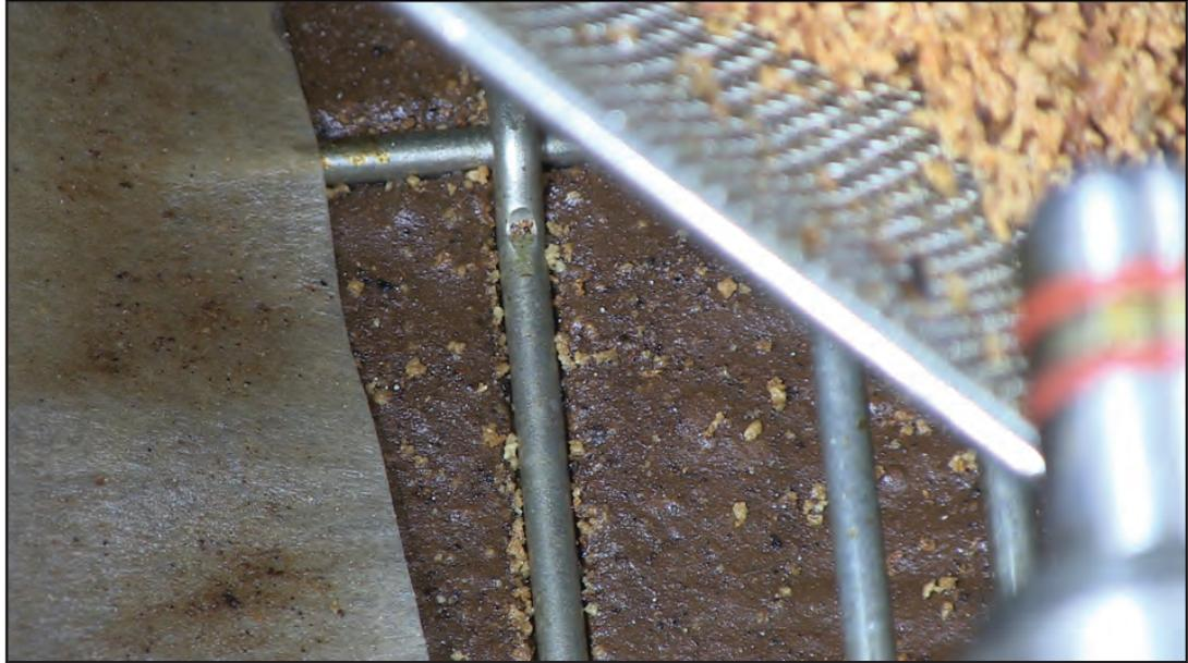
Failure to respond to the fryer's request for filtering leads to oil issues: oil is slow to drain from the pot, oil is slow to return to the frypot from the filter pan. The pump gets clogged. These are often not warranty repair issues and, for that reason, Frymaster requires filter stats be collected on fryers such as the auto-filtering models that collect data.
