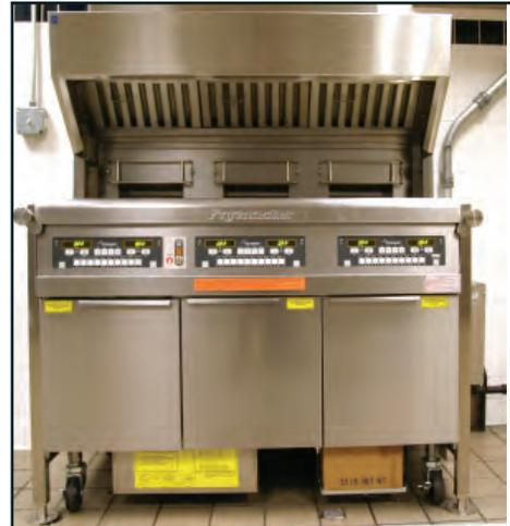
A fryer is shown in a universal hood (above). This installation requires a gas fryer to retain a spacer (below) that is attached at the factory. Installation in a Cap-N-Splash hood requires the removal of the spacer and the Cap-N-Splash locking device must be in place.
