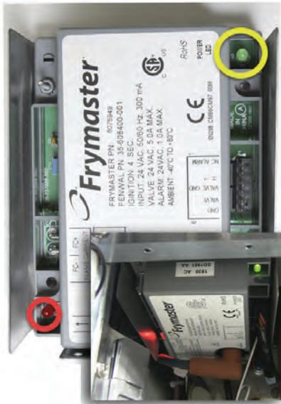
Left module with view of flashing LED in inset.
