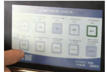
Actuators showing Fault on the Component check screen are likely not receiving power.
