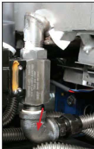
The probes that make the top off and automatic filtering work are shown inside and outside the frypot (above). The oil's movement can be hindered by clogs in the drain elbow (left) in stores that allow crumbs to gather in the frypot.
