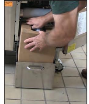
The brace (above) that stiffens the cabinet for transport must be removed and a JIB placed in the cabinet (right) during the setup.
