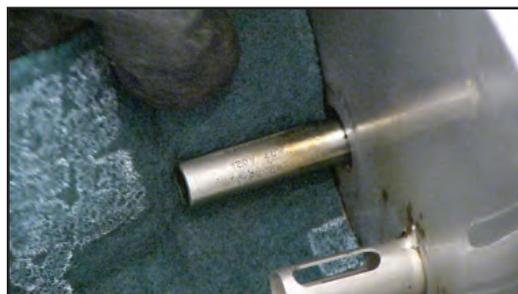
Regular cleaning of the Oil is Back sensor is critical. Insulating oil residue affects its operation and oil won't return to the frypot.
