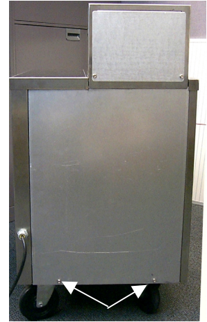
Fig.1: Two screws hold the back in place.
