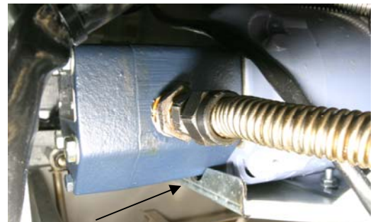
Figure 3: The platform holding the pump must be notched or bent to accommodate the downward facing V-shape of the repositioned pump.
