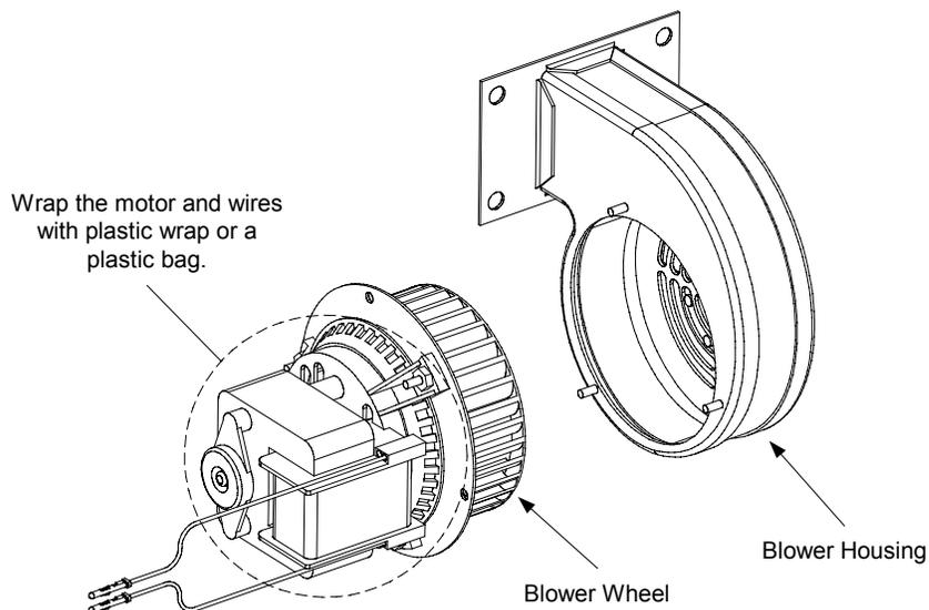
4. Remove the plastic wrap from the blower motor assembly. Reassemble the blower motor assembly and blower housing. Reinstall the blower assembly in the fryer.
