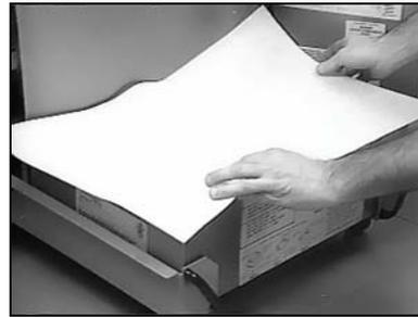
3. Position the hold-down ring over the filter paper and lower the ring into the pan, allowing the paper to fold up around the ring as it is pushed to the bottom of the pan.
