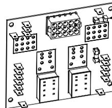
For units in which the ignition module has no fuse, replace the upper fuse on the interface board.
