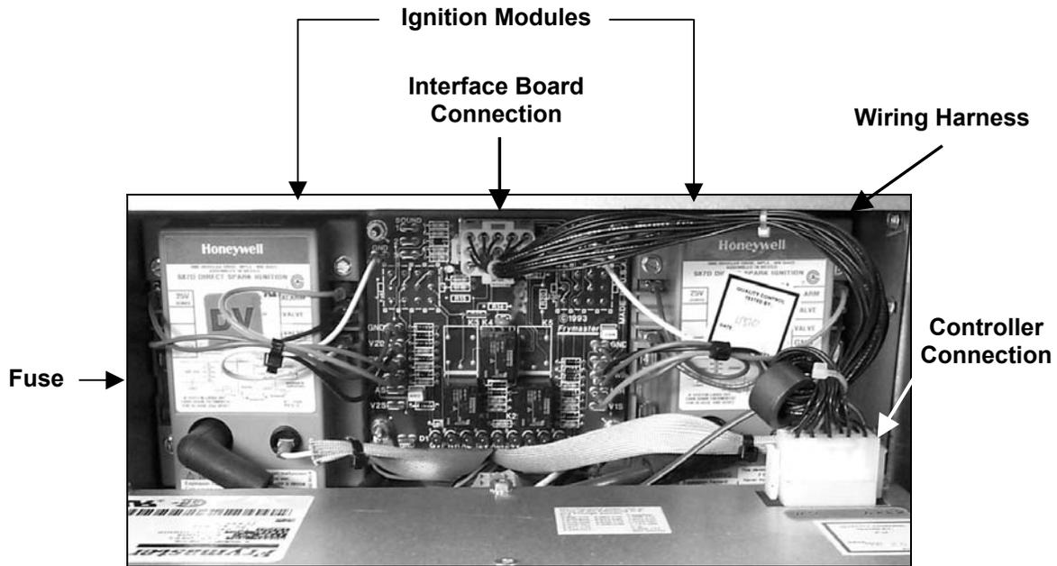
2. Disconnect the wiring harness from the back of the controller and, if replacing the harness, disconnect it from the interface board (see photo on preceding page).
