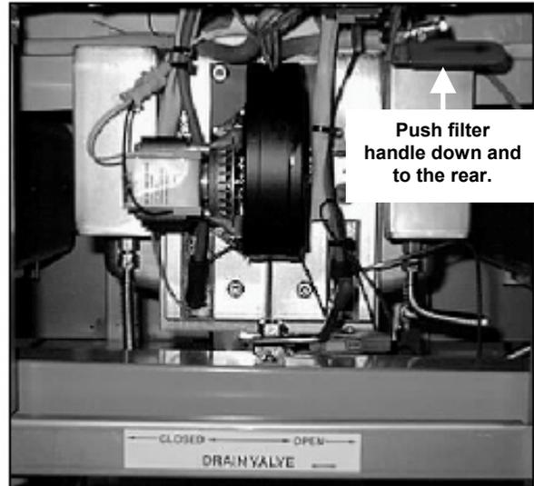
5. After the oil is filtered, close the drain valve and allow the fryer to refill. Let the filter run 10 to 12 seconds after bubbles appear in the oil to clear the lines and prevent hardening or shortening in the lines.
