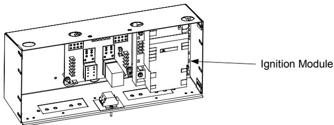
Depending upon when the unit was manufactured, full vat units may have either one or two ignition modules. If there is only one ignition module, the fuse will be mounted on the interface board.
