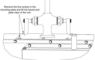
6. Separate the faucet manifold from the remainder of the plumbing as shown in the illustration below.
