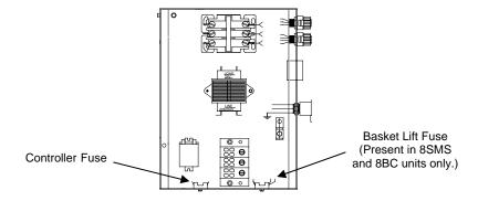
3. Replace the component box cover, being sure to reconnect the ground wire with the upper left screw.
