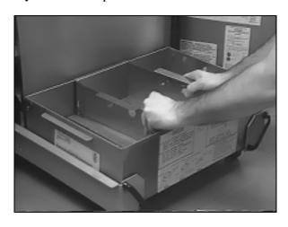
5. Push the filter pan back into the fryer, positioning it all the way to the back of the cabinet. (Some older filter systems have a green HEATER ON indicator, which will light when the assembly is properly positioned.)
