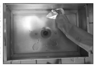
2. After verifying that the metal filter screen is in the bottom of the pan, lay a sheet of filter paper over the top of the pan, overlapping on all sides.
