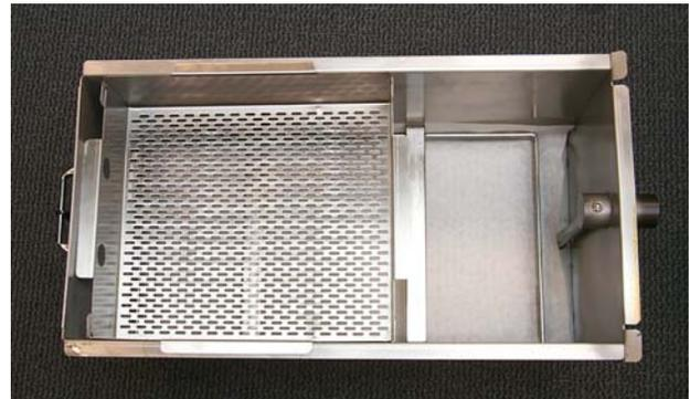
8. Install the filter into the cabinet. Ensure the pan connection securely connects to the cabinet connection. The system is ready for filtering.
