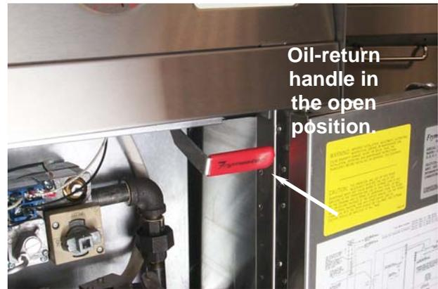
4. Oil will flow through the Power Shower, rinsing debris from the frypot. Continue circulating oil through filter for 5 minutes.
