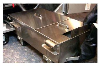
Pull the filter pan from the fryer and remove covers.
