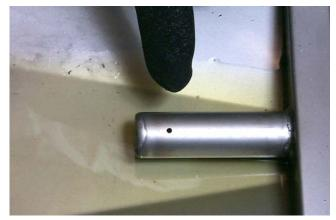
Vent hole location on pickup tube.
