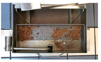
Empty contents of the crumb screen into a fireproof container immediately after filtering is complete.
