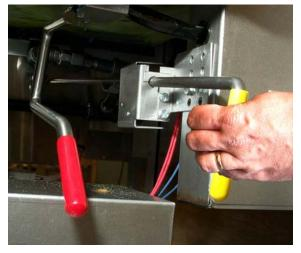
Pull the yellow handle to open the oil return valve and activate the filter pump.
