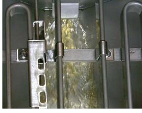
Allow the shortening/oil to circulate the prescribed time period to ensure all sediment and suspended particles are removed.
