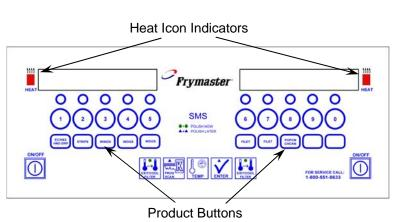
At 255°F (124°C), the computer will display actual temperature until setpoint temperature has been reached. When the fryer comes out of melt cycle, the fryer will go into continuous heat mode until the setpoint temperature is reached. When the computer calls for heat, heat icons will light while the heating elements are energized. At setpoint temperature, the computer will display "DROP".
