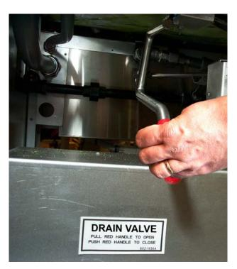
Pull the red handle to open the drain valve.
