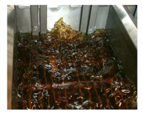
Allow the shortening/oil to bubble for 10-15 seconds to ensure evacuation of all shortening/oil in the return lines.
