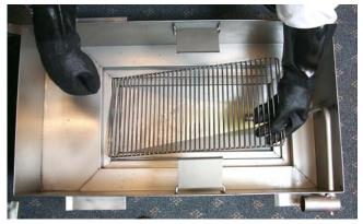
Remove filter screen from filter pan.
