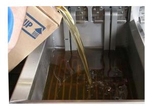
Add oil/shortening until the oil level is at the top OIL LEVEL line. DO NOT OVERFILL THE FRYPOT.
