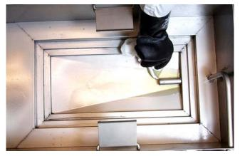
Clean filter pan and all pan components. Ensure all parts are thoroughly dried before reassembly.
