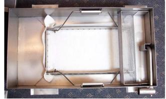
Properly assembled filter pan, ready for use.
