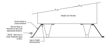
NOTE: The installation must be inspected after it is complete to ensure it meets the intent of these instructions. The on-site supervisor and/or operator(s) should be informed that the appliance is installed with restraints. If restraints are removed to move fryer (cleaning beneath and behind, relocation, etc.), ensure that they are re-installed when fryer is returned to its permanently installed position.
