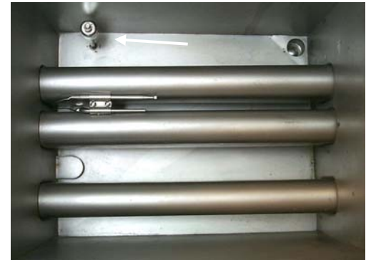
Cook vessel and lower float switch (arrow).
