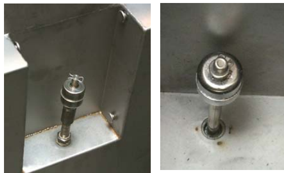
Figure 1: The float switches (above and right) should be cleaned periodically to eliminate starch buildup, which can impede the motion of the floats. Care must be taken, however, to ensure the shafts are not dislocated or the movement of the float hindered.
