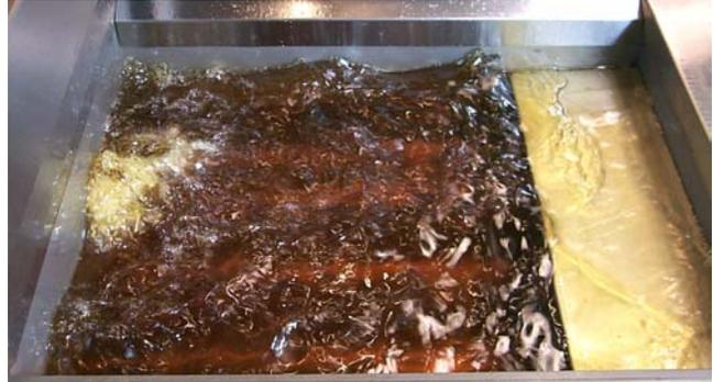
Allow the shortening/oil to bubble for 10-15 seconds to ensure evacuation of all shortening/oil in the return lines.
