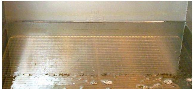
Add oil/shortening until the oil level is at the top OIL LEVEL line. DO NOT OVERFILL THE FRYPOT.
