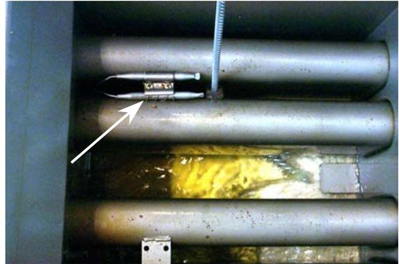
Clean all sediment and suspended particles from the burner tubes and frypot as the oil begins to circulate. Use care not to disturb the probes (arrow) on the burner tube.
