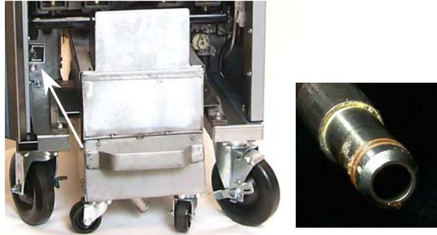
The filter pan slides under the fryer (left), connecting with a slip fitting (right). [Note location of filter by-pass switch and filter reset breaker (arrow)].
