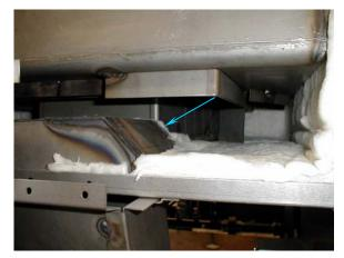
Ensure blower-housing insulation strip remains in place after installing the new frypot (arrow).
