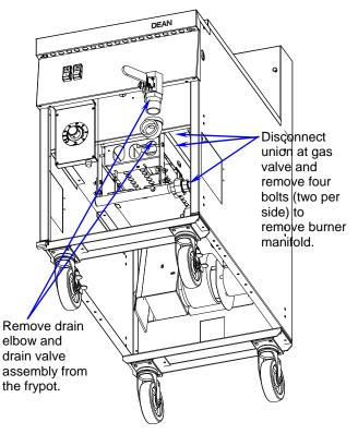
Disconnect union at gas valve and remove four bolts connecting burner manifold brackets to firebox, elbow and drain valve assembly from frypot.
