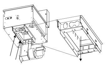
After removing burner-box baffle, remove screws (two) securing the flame spreader to the burner box. Allow the flame spreader to drop down in the burner box to clear the frypot baffles. Repeat for both sides.
