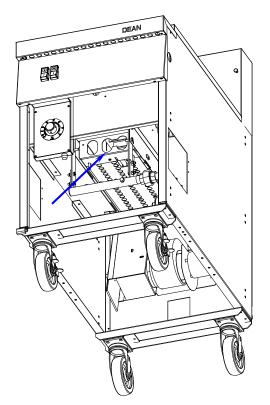
Inspect frypot baffles through burner tube opening (arrow) for signs of burn-through or damage.
