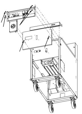
Remove topcap, wireway box and front heat shield to access firebox and frypot.
