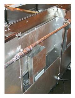
Multi-batteried systems after 02/03 have upper and lower back panels, which must be removed to access the blower assembly (fryer above shown with upper back panel removed).
