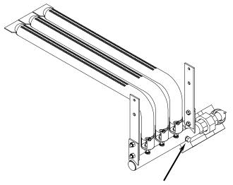
Remove pressure tap from burner manifold to check burner manifold pressure.
