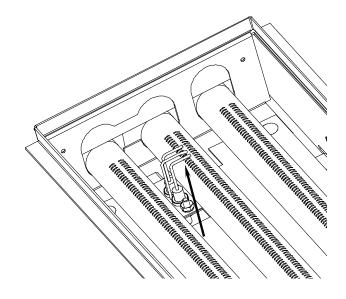
Ensure ignitor is properly positioned (arrow) over the center burner prior to tightening the mounting screw.
