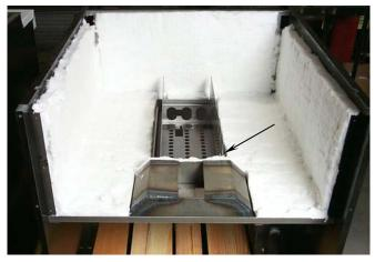
Install new insulation in firebox using spray adhesive, ensuring good contact between insulation and metal surfaces.
