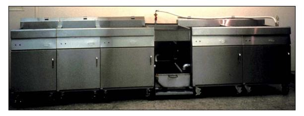
The first generation filter returned the shortening to the frypot using a hose and wand assembly. Later versions used a so-called "hands free" plumbing assembly attached to the backsplash of the dump station.
