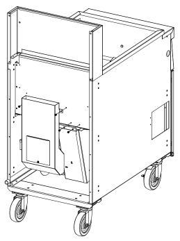
After removing screws (arrows), remove blower assembly from firebox by pulling outward.
