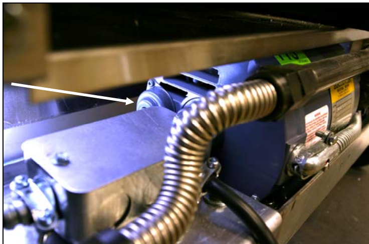
Filter Pump Reset Switch (Arrow)
