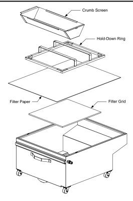
4. Push the prepared filter pan back into the fryer cabinet and reconnect the suction hose to the pan.
