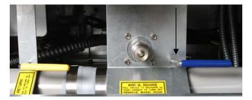
The handle (above, see arrow) next to the oil-disposal quick-disconnect activates the filter pump. All drain valves should be closed when oil is being pumped out for disposal.
