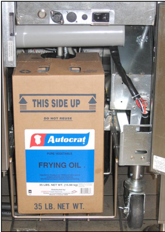
The reservoir, or JIB, rests behind the right door of the fryer. A light on the front of the fryer illuminates when the jug is empty.
