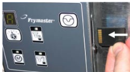
Insert the SD card with contacts facing the front of the fryer.
