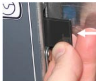
Remove the SD card using the fingernail slot on the top of the card.
