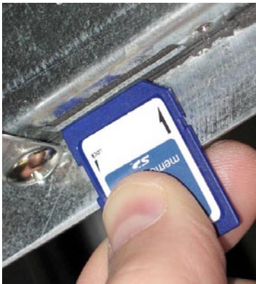
Insert the SD card with contacts facing up.
