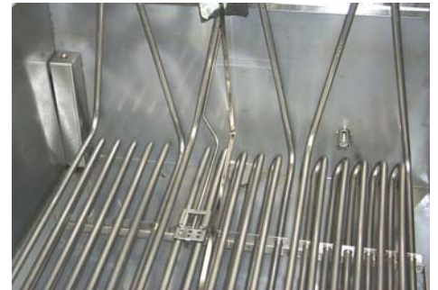
The earlier 2836 units have round heating elements and a float switch, which is visible in the left corner above.
