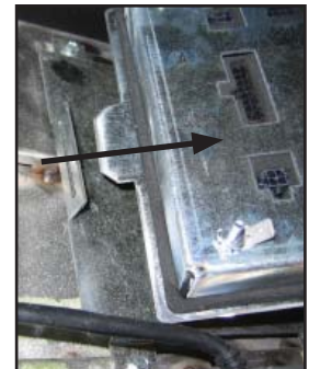
The bottom tab slides out of the bracket attached to the frypot.
