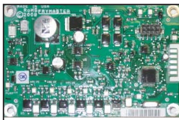
The ATO board positioned underneath the LON gateway controls the top off of the fry pots.
