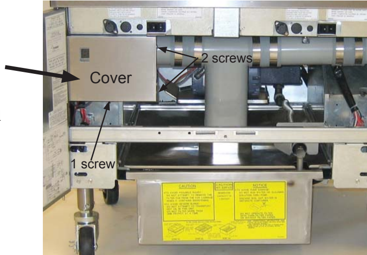
MIB controller cover (three screws hold it in place).
