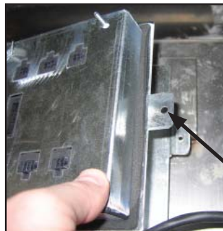
After removing the screw, the AIF assembly drops down.
