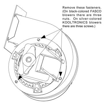
4. Wrap the motor with plastic wrap to prevent water from entering it. Spray degreaser or detergent on the blower wheel and the blower housing. Allow it to soak for five minutes. Rinse the wheel and housing with hot tap water, then dry with a clean cloth.
