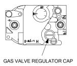
7. Place the power switch and the gas valve in the **OFF** position. Remove the fitting from the pressure tap hole and reinstall the pressure tap plug.
