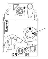
2. Remove the pressure tap plug from the gas valve assembly.
