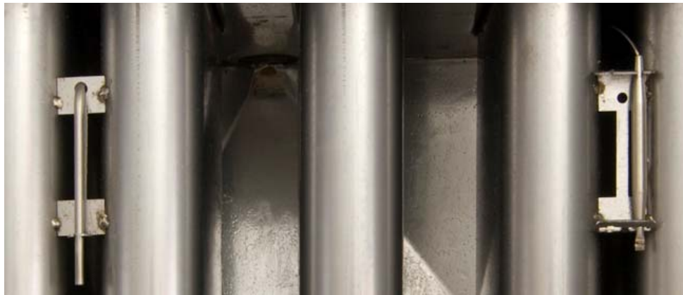
Typical sensor probe/high-limit locations and mounting hardware.
