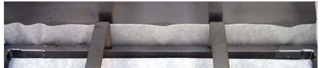
Ensure filter paper overlaps two inches on all sides and is evenly distributed under the hold-down ring.
