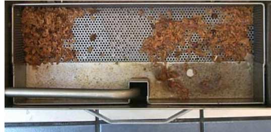
Empty the filter pan crumb tray into a fireproof container at the end of frying operations each day. DO NOT ALLOW CRUMBS TO ACCUMULATE IN TRAY.
