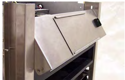
Fig. 3. Removing front fascia.
