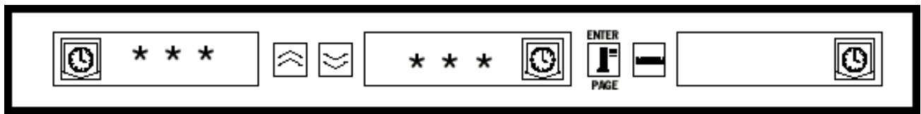
Fig: 15: In the test mode, asterisk-like symbols will illuminate in the displays, appearing to march from display to display from left to right. In units with rear displays, this light motion is repeated on the rear displays.
