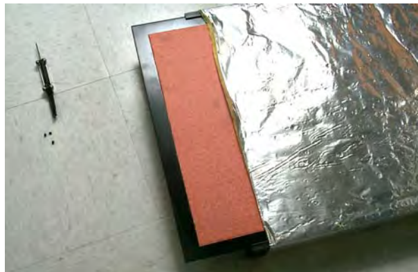
Fig. 20. Slide the loosened heater plate from the spacer.
