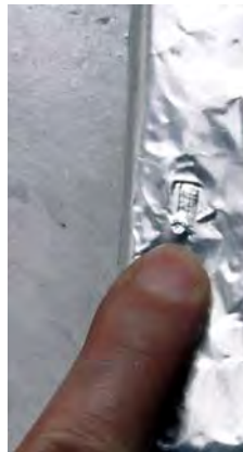
Fig. 18. Locate setscrews under heater plate covering.
