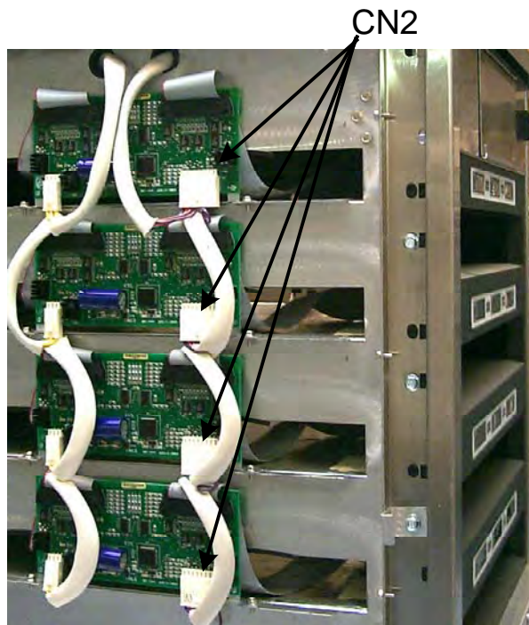
Fig. 14. CN2 connectors are disconnected from the driver board to test new displays.
