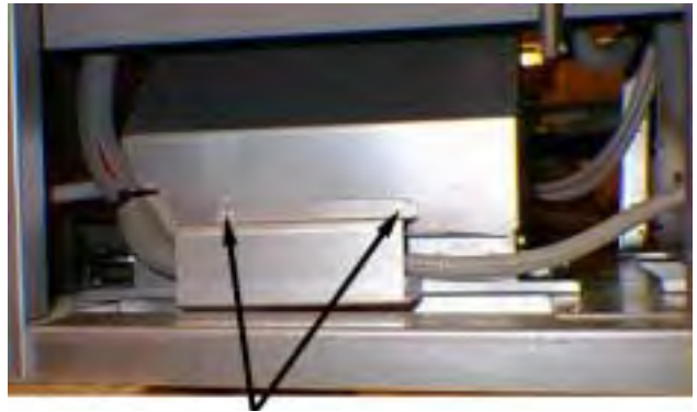
Screws securing wire cover to contactor box (optional on old-style contactor boxes)
