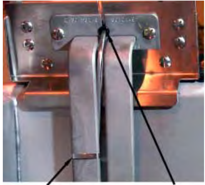
Secure probe to element with metal Ty-Wrap
