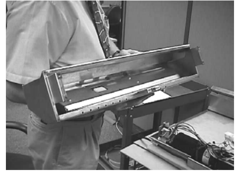
The cowl assembly is held on by five screws, which are removed from the bottom of the unit.
