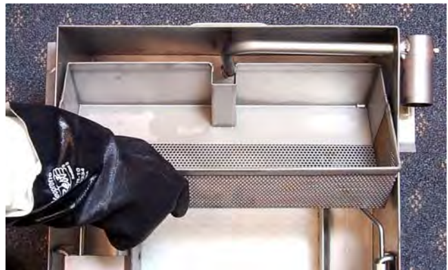
Remove crumb screen. If crumbs are present in the crumb screen, empty the screen into a fireproof container. Wash the screen in hot, soapy water, rinse, then dry thoroughly.
