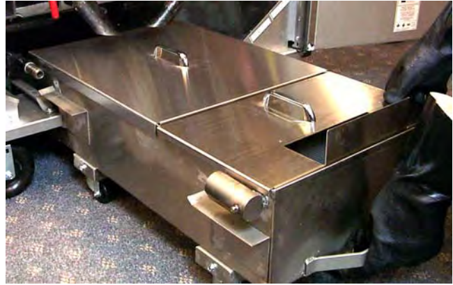
Pull the filter pan from the fryer and remove covers.
