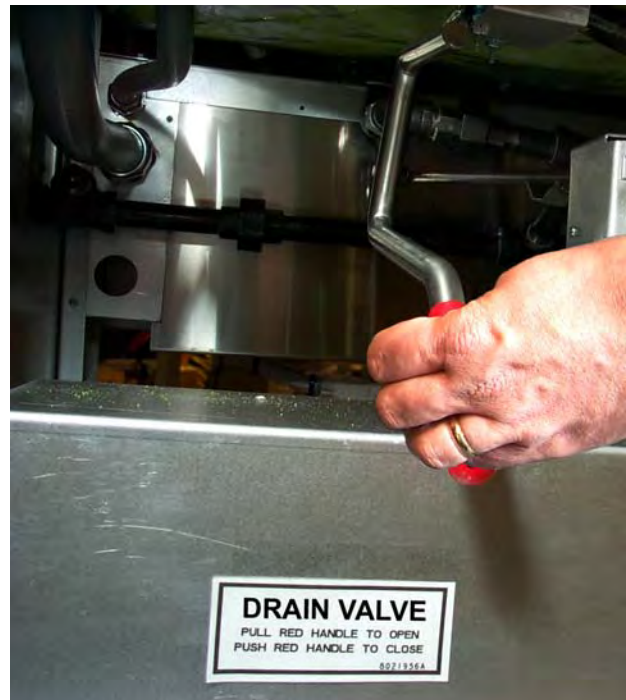
Pull the red handle to open the drain valve.
