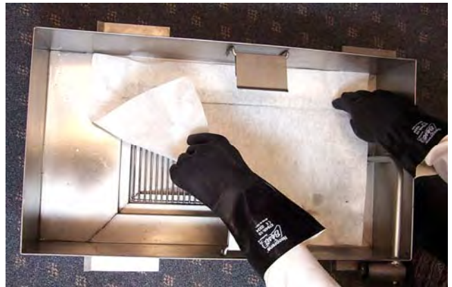
Remove and discard old filter paper.
