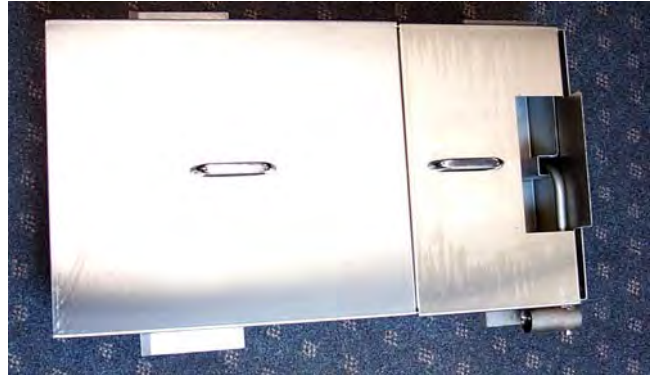
Pan covers properly placed.
