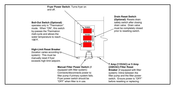
**FRYER POWER SWITCH** – This switch turns the fryer on and off. When the power switch is in the "ON" position, the indicator light will be lit when calling for heat.
