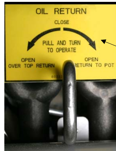
Pull and turn the oil return handle to open the oil return valve and activate the filter pump.
