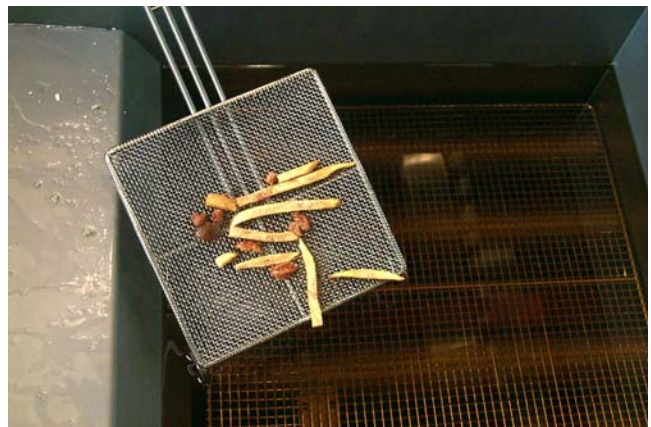
Remove large debris from frypot prior to filtering.
