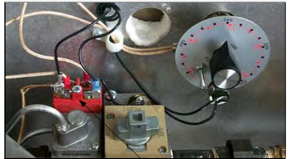
Step 3: Mark and disconnect the wires from the gas valve.
