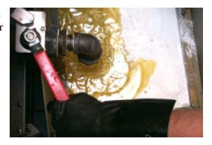
10. Allow the pump to run for 10-15 seconds after air starts to flow through the wand, before shutting off the filter. Clearing residual shortening/oil from the return lines reduces the likelihood of clogged lines.
