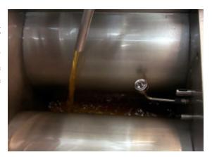
9. Close the drain valve handle. It takes approximately 5 to 7 minutes for the filter to pump all the oil back into the fryer.
