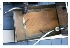
Scrape excess sediment from top filter paper sheet after filtering.
