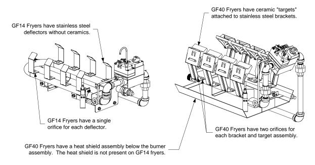
The flames originate from orifices in a U-shaped burner manifold positioned beneath the frypot. The orifice diameters differ for natural and Propane (LP) gas and for fryers as indicated in the accompanying table (NOTE: This table shows only the orifices used in elevations up to 1999 feet/609 meters. See Chapter 2 (GF14) or Chapter 3 (GF40) for orifices required at other elevations). GF14 fryers have one orifice per deflector; GF40 fryers have two orifices per deflector assembly.
