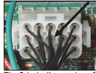
Pin 8 is in the center of the plug. (See arrow).
