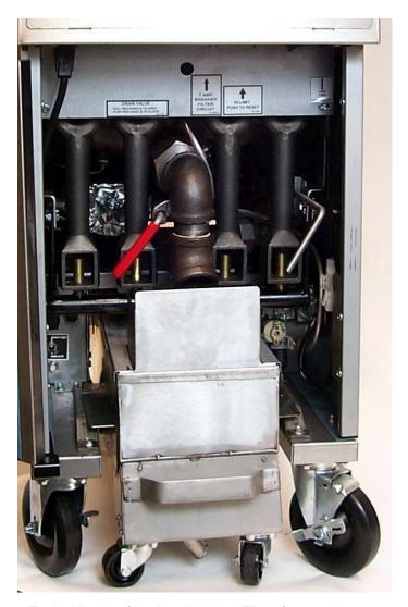
Typical built-in filter installed in a TB14 fryer unit.
