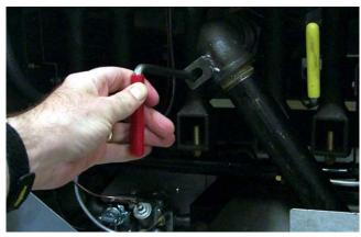
After filtering is complete, close the red drain handle to start refilling the frypot.
