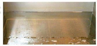
Add oil/shortening until the oil level is at the top OIL LEVEL line. DO NOT OVERFILL THE FRYPOT.
