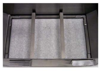
Hold-down ring positioned correctly over filter paper in filter pan.
