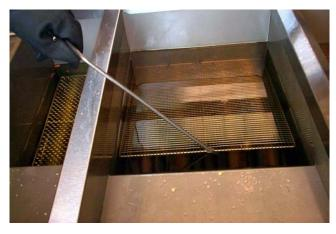
Removing support grid from frypot prior to filtering.
