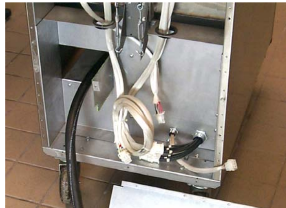
Ensure element wire insulation is installed and that the wires are properly routed to prevent wire chafing.
