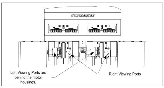
The optimum burn is a bright orange-red glow. If a blue flame is observed, or if there are dark spots on a burner face, adjust the air gas mixture as follows: On the side of the blower housing opposite the motor is a plate with a locking nut. Loosen the nut enough to allow the plate to be moved, then adjust the position of the plate to open or close the air intake opening until a bright orange-red glow is obtained. Carefully hold the plate in position and tighten the locking nut.
