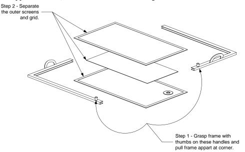
2. Separate the outer screens and grid.
