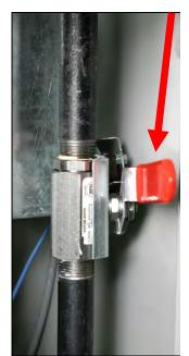
Earlier oil discharge valve handle is shown in the OFF position. Push down to discharge oil from the filter pan.
