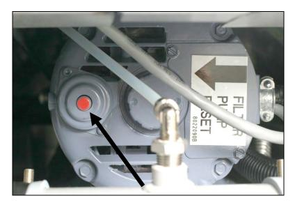
Filter Pump Reset Switch
