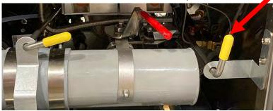
Later oil discharge valve handle is shown in the OFF position. Pull to discharge oil from the filter pan.
