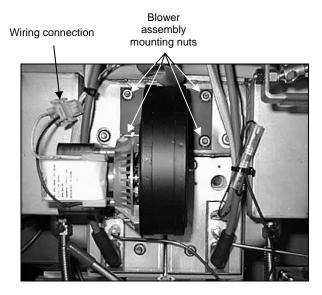
2. Remove the three fasteners that secure the blower motor assembly to the blower housing, and separate the two components.
