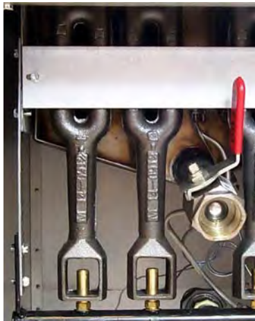
Typical frypot drain valve (SM40 shown).
