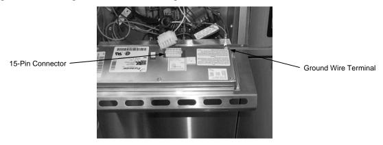
3. Remove the controller from the control panel assembly and install the replacement controller. Reinstall the control panel assembly by reversing steps 1 and 2.
