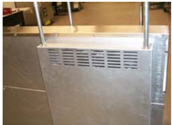
Install the cabinet backs, basket lift assembly, and top cap after probe installation is complete.
