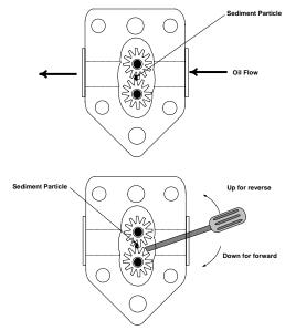
be freed by manually moving the gears with a screwdriver or other instrument.
