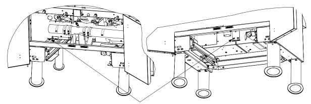
Remove these screws to dismount the left contactor box. The right contactor box is secured in a similar manner.
