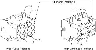
be Lead Positions High-Limit Lead Position
