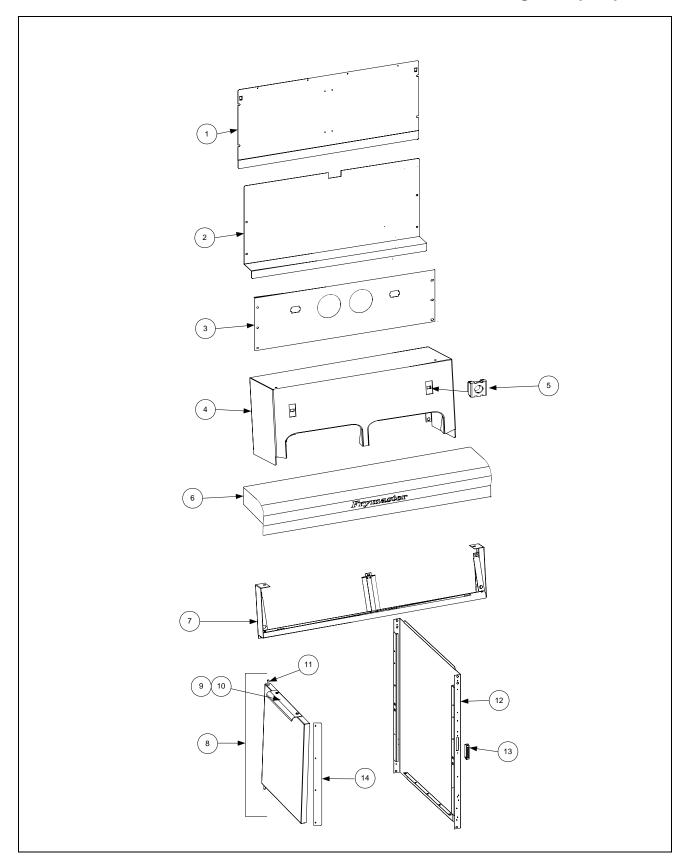
8.2.1 FPPH217 Backs, Panels, Doors, Handles, Sides, Tilt Housings & Top Caps
