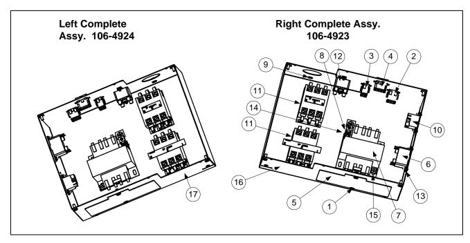
**NOTE 1:** Left and right contactor box assemblies are mirror images of one another. With the exception of the box itself, all components of a left-hand assembly, including the lid, are the same as those in the corresponding right-hand assembly and vice versa.
