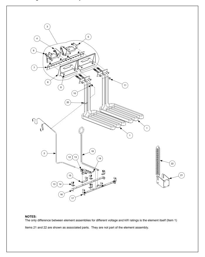
8.4.3 Heating Element Assembly and Associated Parts cont.
