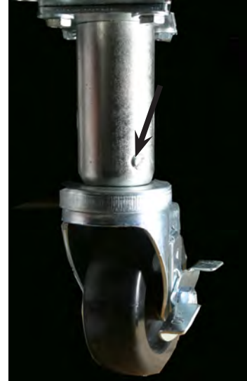
Arrow points to setscrew on front caster.
