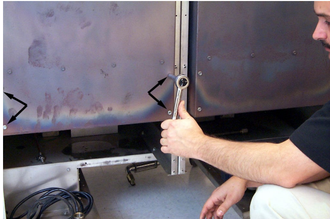
Removing bolts (arrows) securing flue to cookpot.
