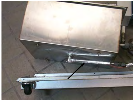
Remove foil-insulating tape to expose heater strip (arrow).
