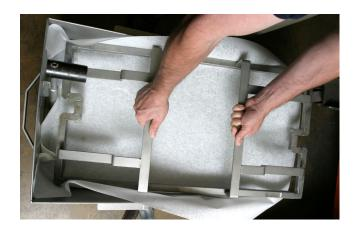
4. Remove and discard old filter paper sheet from the filter pan.
