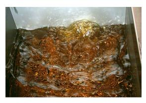
8. Turn off the filter by turning the oil return handle to the left, into the CLOSED position. This closes the oil return valve under the filtered frypot and stops the filter pump motor.
