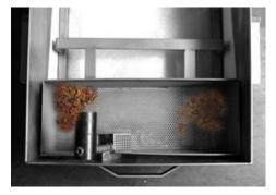
Empty contents of the crumb screen into a fireproof container immediately after filtering is complete.
