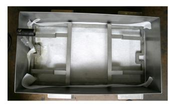
10. Sprinkle 1 cup (8 ounces/27 grams) of filter powder evenly over the paper. Use a measuring cup or scoop to evenly distribute filter powder over the filter sheet.
