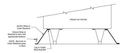
**NOTE**: If you need to relocate a fryer installed with legs, remove all weight from each leg before moving. If a leg is damaged, contact your service agent for immediate repair or replacement.
