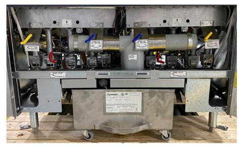
The levers on the right and left of the cabinet return oil through rear ports in the frypot. The center-mounted levers return oil through a top-mounted faucet. In all cases, a yellow or blue lever returns oil to the frypot directly above it.
