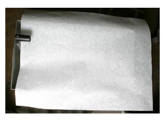
9. Reinstall the hold-down ring. Ensure filter paper is properly aligned under the hold-down ring. Press the filter paper into place with the hold-down ring, ensuring the paper laps against the walls of the filter pan.
