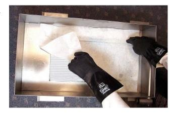
5. Remove the filter screen from the bottom of the pan.
