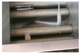
Use the L-shaped brush to loosen debris as oil drains from the frypot.
