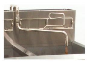
• Over-the-top Oil Return: Allow the faucet to sputter for 15-30 seconds to ensure the oil return lines are clear of oil.
