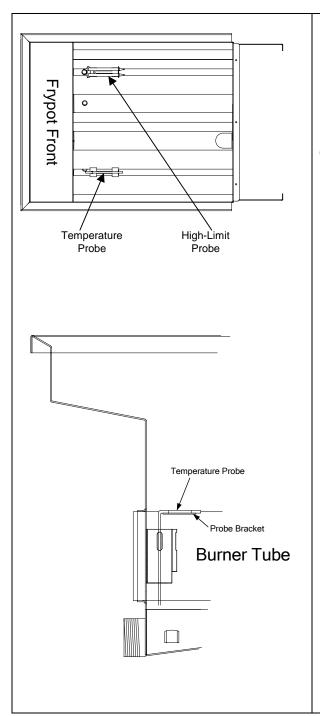
No: Ensure the probe tip is ½" from the top of the burner tubes (see illustration). If the probe adjustment is correct, the controller probe circuit may be faulty. If probe adjustment is incorrect, it will require adjustment.
