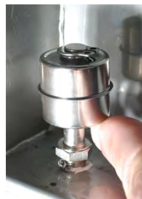
High-level float switch
