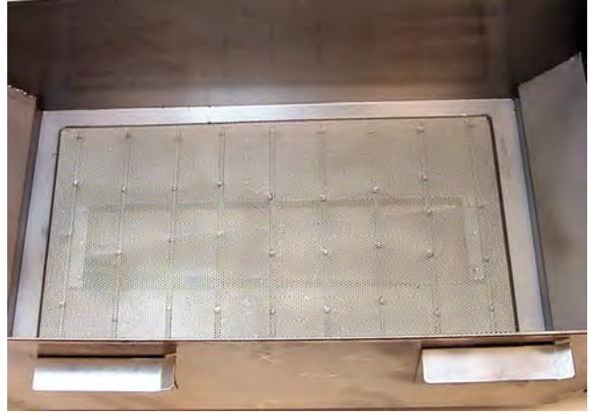
Support grid properly placed in filter pan.
