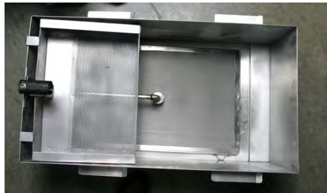
Remove the crumb screen by lifting it up and out.
