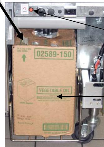
**F: JIB reset button:** Press and hold after replacing the JIB until yellow light goes out..
