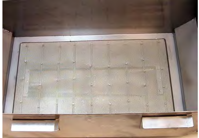
Support grid properly placed in filter pan.
