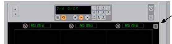
Pressing the row mode button (see arrow) produces a sequence of menu choices. With the desired menu for the row displayed, press the OK button on the top keypad.
