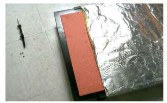
Fig. 13: The heater plate slides from the insulation.
