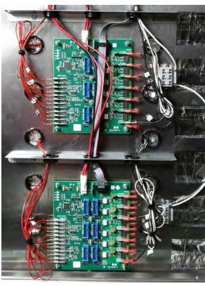
**Fig. 7**: Distribution board shown with display cables removed.
