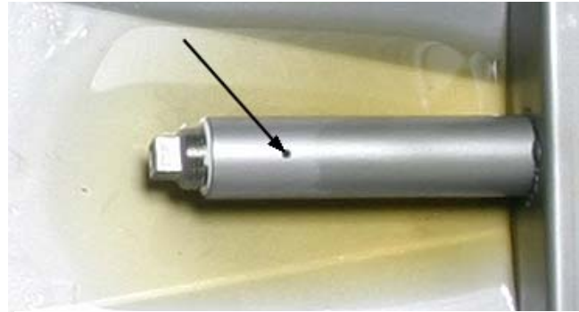
Vent hole location on pickup tube.
