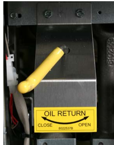
Moving the yellow handle to the open position opens the oil return valve and activates the filter pump.
