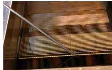
Removing basket support rack from frypot prior to filtering.
