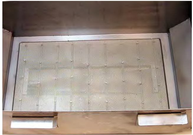
Support grid properly placed in filter pan.
