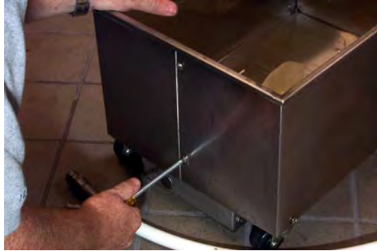
Remove screws securing outer panels.
