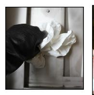
**11A**: Clean the filter pan and reassemble: perforated metal screen in first, filter paper in second, then holddown ring and crumb tray. Change filter paper after each filtering. See Pan Assembly illustration at right.
