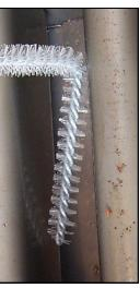
5A: Carefully brush debris from the pot into the flowing oil.
