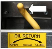
3A: Open the yellow-handled oil return valve. The filter pump comes on and oil flows from the filter pan to the frypot and back to the pan.
