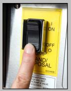
9B: Turn off the wand when the frypot is full. 10B: Close the Wand/Disposal valve. 11B: Remove, drain and store the wand/disposal hose. **12B:** Clean the filter pan as shown in step 9A through 12A below.
