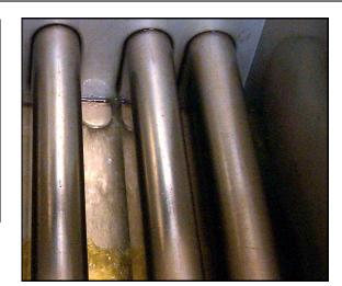
**4A:** Oil flows through the frypot and out the open drain valve.
