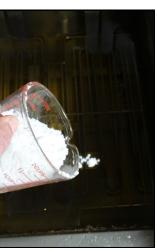
12A: Add one cup of Magnesol to the filter pan or to oil in the filtered vat.
